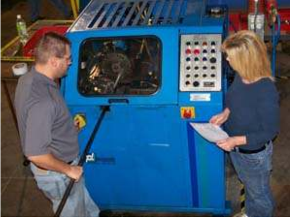
Traci Kramer (right) and Josh Hairell of Harco use a Wauseon end forming machine to produce tube flaring and other tube end forms.
